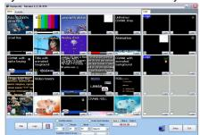
channel – 4 independent layers, static or animated logo, digital and analog clocks, digital timer, crawling, rolling, title's effects, video up to full screen, banners. All functions can be controlled by the remote control panel. GPI input allows to turn off graphic by external device. Graphic pages are prepared with TEXTUS EDITOR software. Pages are loaded into TEXTUS AIR windows and are ready to go on air imediately, either by mouse clicking or pressing a key on the remote
